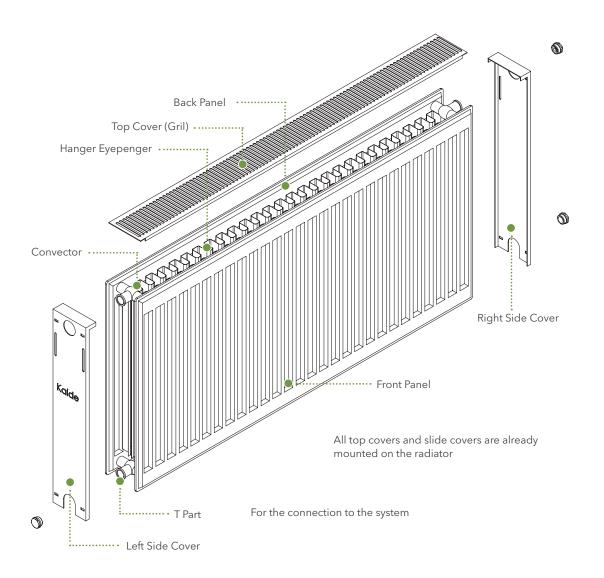
Both the radiator's inner and outer surfaces are fully cleaned and purified by dipping, spray oil taking, phosphatizing and passivization conforming to DIN 55900. As a result, the whole surface of the radiator is totally purified from any chemical substances that might effect the quality of the paint. A premier coating is applied by dipping. The radiators then pass through a furnace, and are painted in climatized cabinets by robotic pistols with electrostatic powder paint and are furnaced again.
