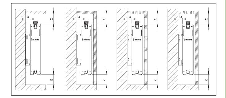
The efficiency changes depending on how the radiator is covered can be seen from the figure.
