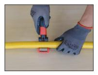
Cut the inflex hose properly with a special cutting scissors (without burr and deformation at the end of the hose). Twist the scissors around the hose, tightening a little more each turn.
