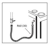
1- Please install the N-Gas hose according to written limits on the hose. Please choose the suitable hose between gas valves and gas burner device. Unpack the hose only when you are going to connect it to the installation.
