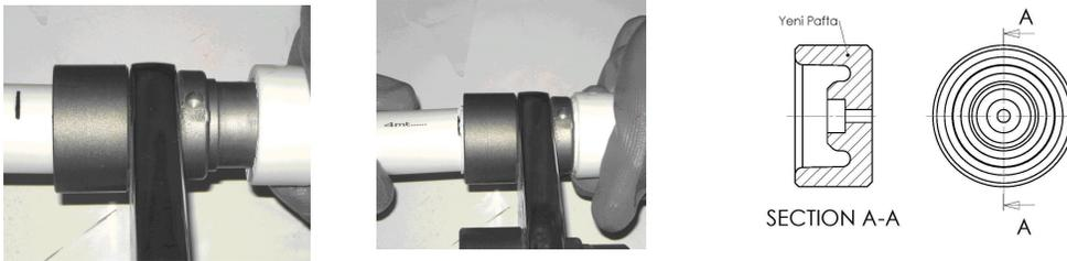
3. Before welding be sure that pipe has a circular form at the front face and foil covered well with melted inner and outer layers of the pipe.
